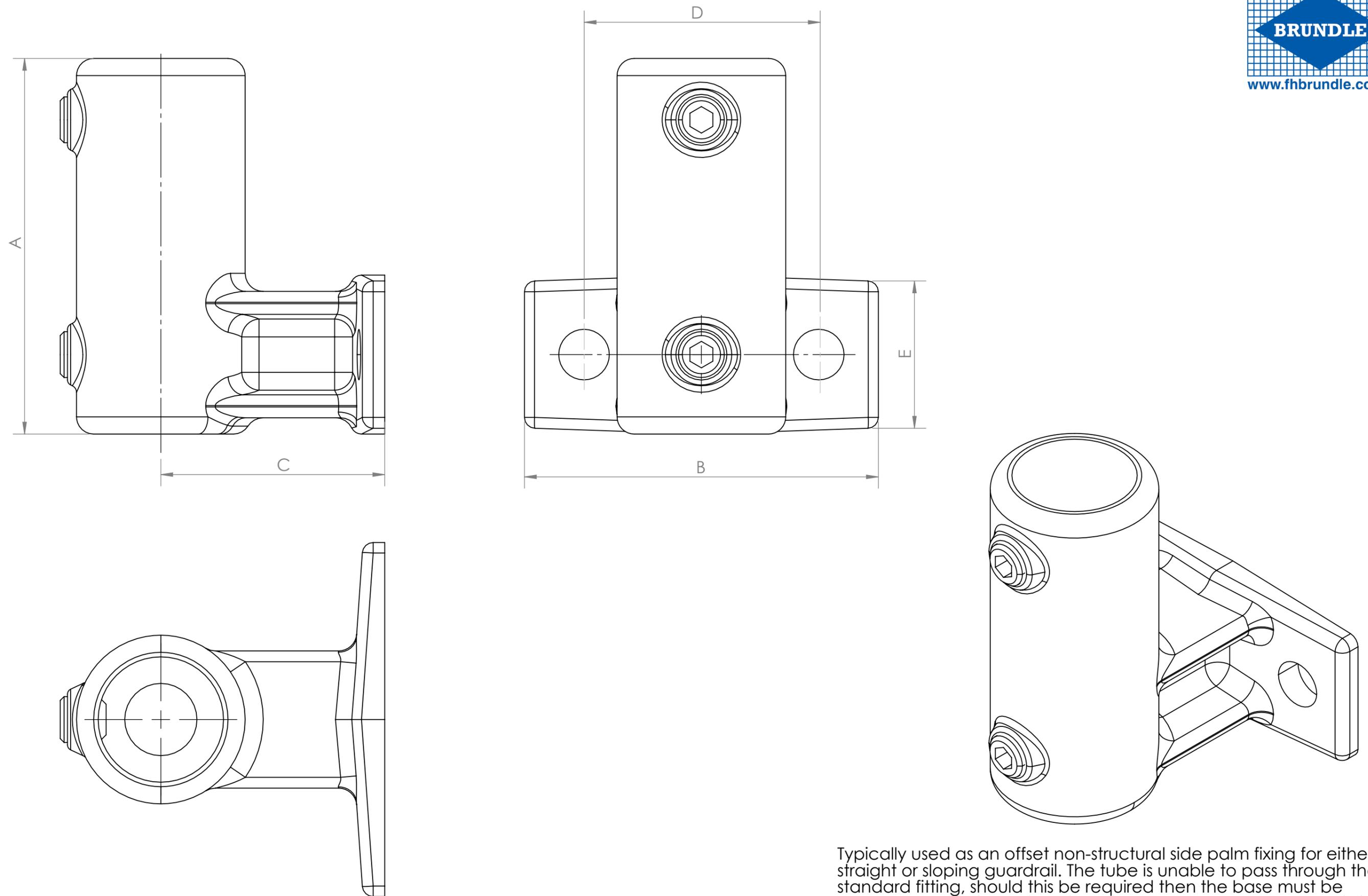
Typically used as an offset non-structural side palm fixing for either straight or sloping guardrail. The tube is unable to pass through the standard fitting, should this be required then the base must be reamed out. Use in conjunction with a 143 when a secondary inline base fixing is required.
